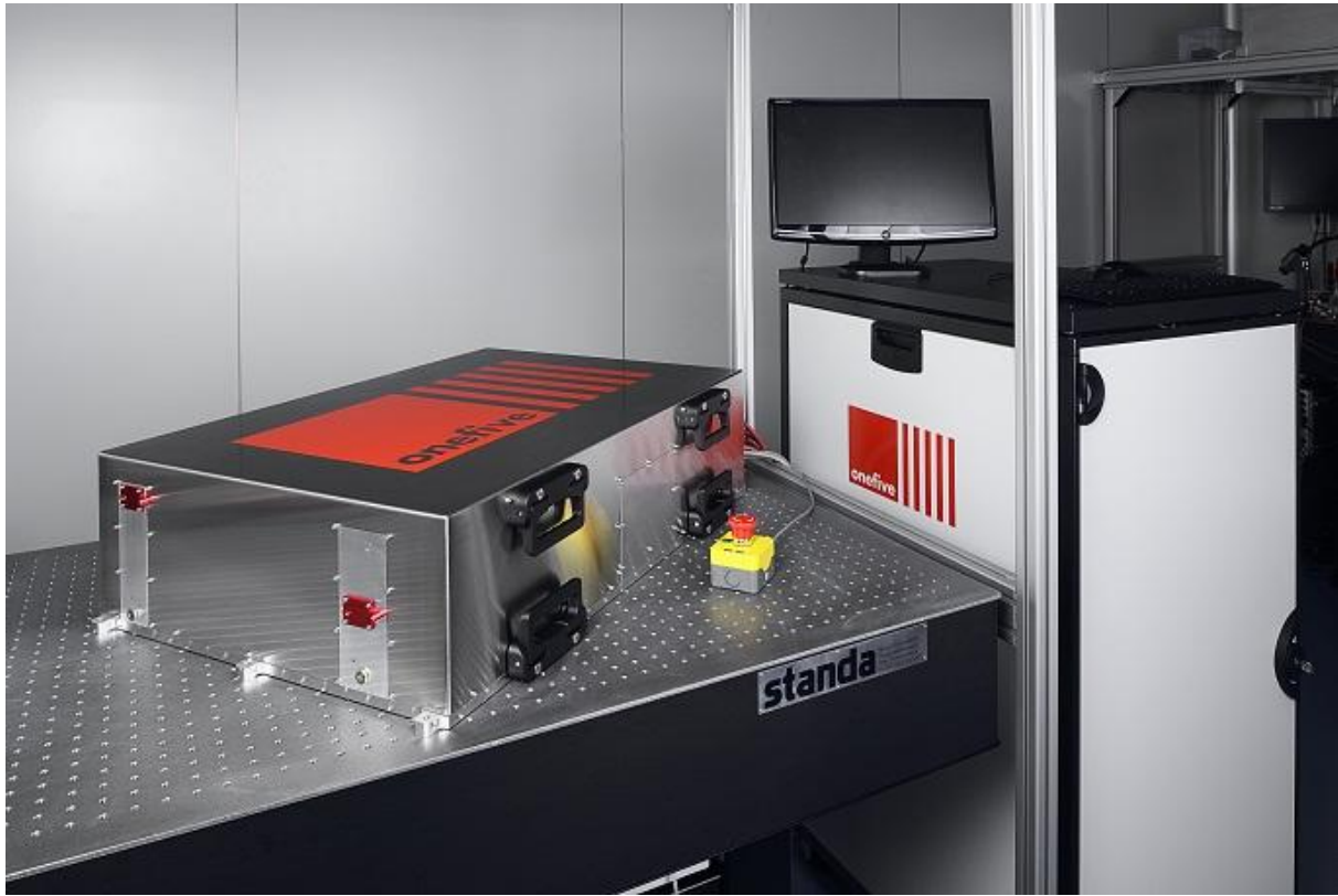
Fig. 1: The air-cooled Origami - 10 XP Dual Burst laser featuring the dual output for simultaneous seeding and pumping of a non-collinear optical parametric amplifier installed at the European XFEL.
